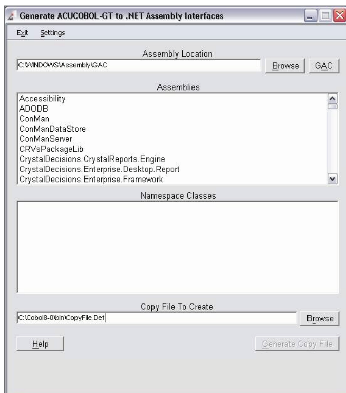
Figure 3: .NET and ActiveX Definitions Generator ACUCOBOL GT includes utilities that generate COBOL FDs and SELECT statements from .NET assemblies and ActiveX controls.
